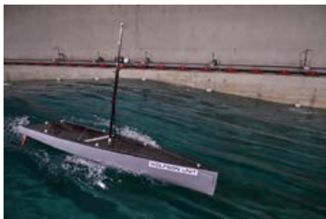
Fig. 8 Motion capture experiments on a free-running sailing yacht (13)
