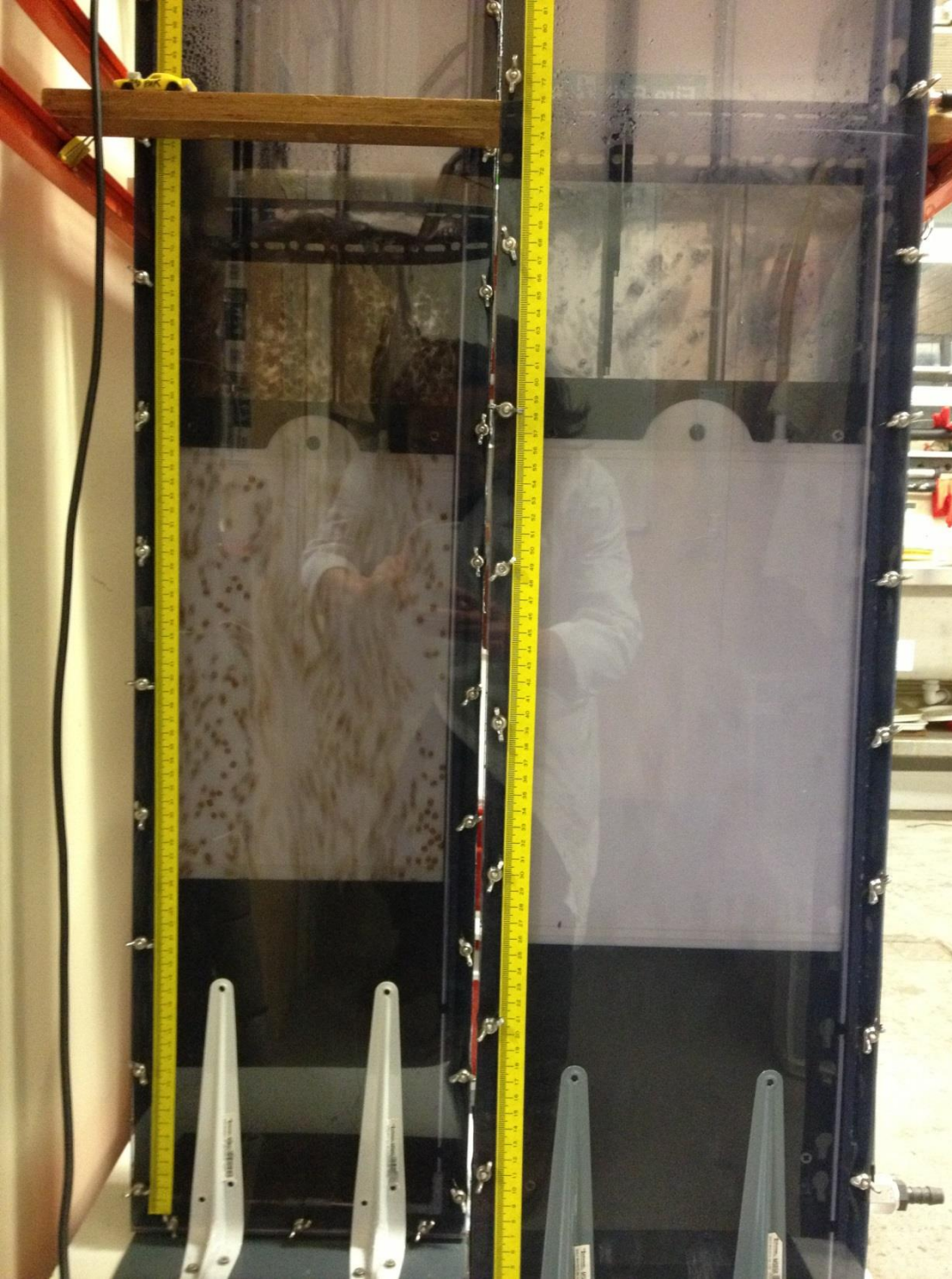
Gas-sparged AnMBR with and without particle addition
