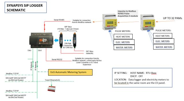
5.3.8 Synapsys Solutions Ltd, Tel: 01444 246 128, shall be commissioned to carry out the programming and connection of the SIP + EMT-IF data logger to the University's Automatic Metering System (AMS). To enable the data logger to be programmed the contractor is responsible for providing
