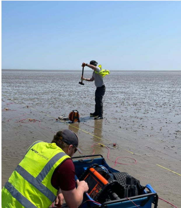
Emily – Work experience conducting seismic refraction surveys for the National Grid.
