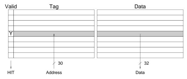
On storage the address and data of an item are stored at any empty location in the memory. The valid flag is set to indicate that the location contains valid data.
