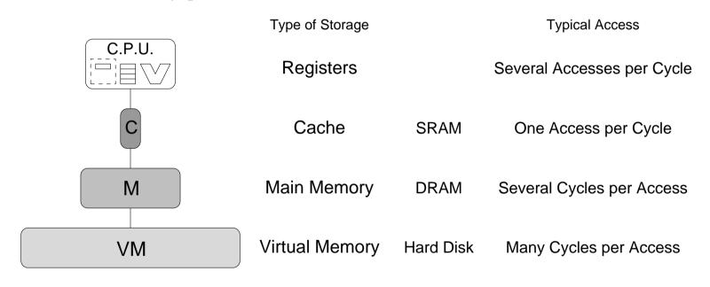
The solution is a hierarchy of memory containing some large components and some fast components.
