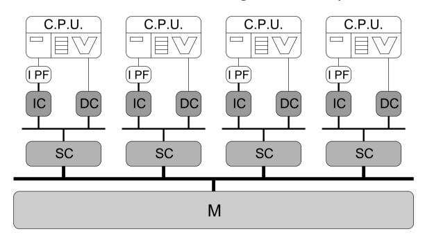
Using the full range of caching techniques available, we can balance the Processing Power and Memory Bandwidth of small bus based systems.
