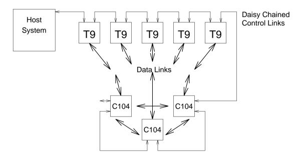
Note that only one C104 is required in order to provide an indirect network with a diameter of 2 for 32 T9000s - although 4 C104s would do the job rather better.
