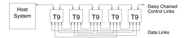
As with the T800, any direct network which requires node valencies of up to 4 can be assembled using T9000 components<sup>2</sup>.
