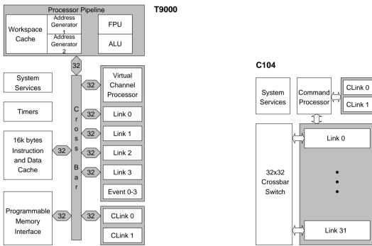
In addition a hardware routing engine (C104) supporting *wormhole routing* over 32 links can be used to create large indirect networks.
