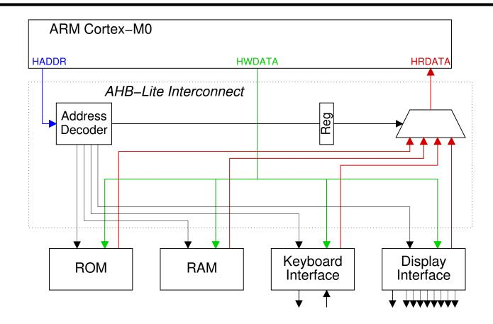
• The Address Decoder controls the multiplexer via a register which adds a single cycle delay
