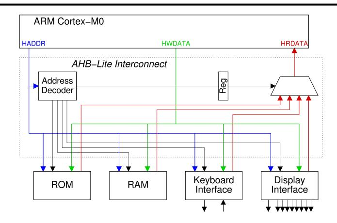
• The low order bits of HADDR are used to select registers within the slaves
