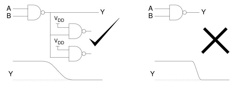
Where a NAND gate is used as the load, tie unused inputs to  $V_{DD}$ . Where a NOR gate is used as the load, tie unused inputs to GND.
