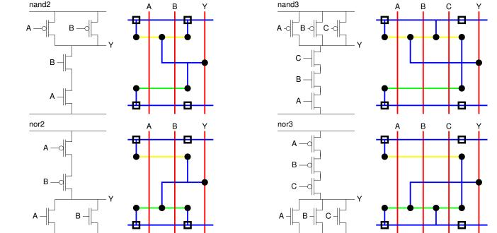
Optimize the gate for equal average rise and fall times based on restrictions you are given<sup>2</sup>.
