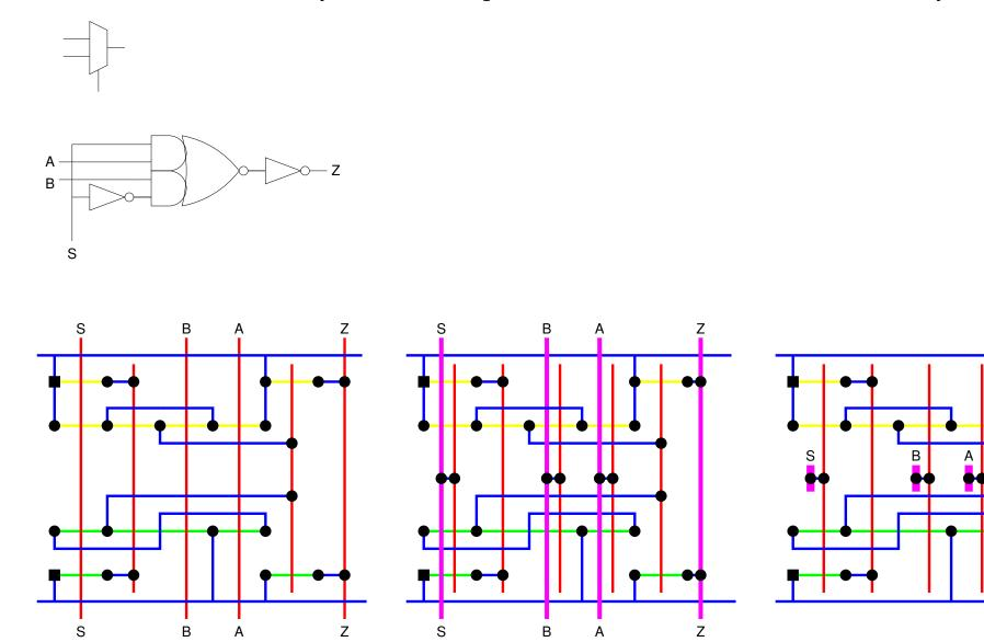
Gate Matrix Style Mux – (for processes with one, two or three metal layers)
