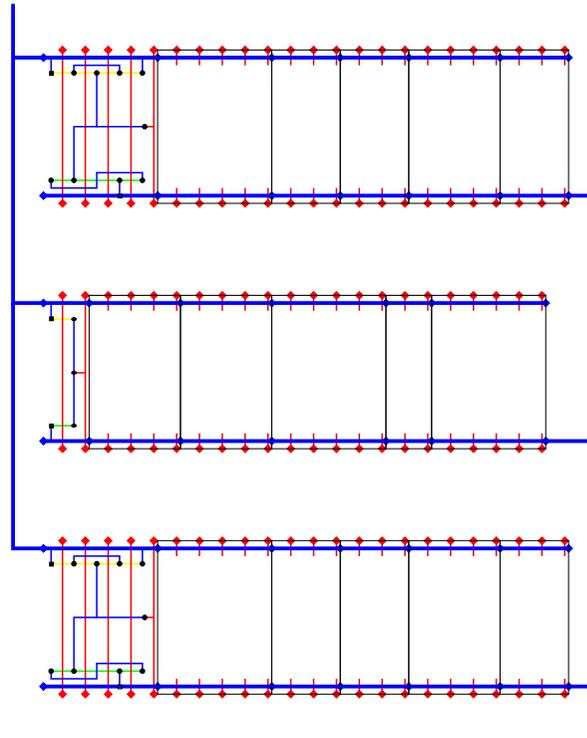
Inter-digitated power and ground rails can be routed using only one metal layer.<sup>2</sup>
