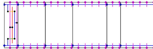
Cells are placed in one or several equal length lines with inter-digitated power and ground rails.
