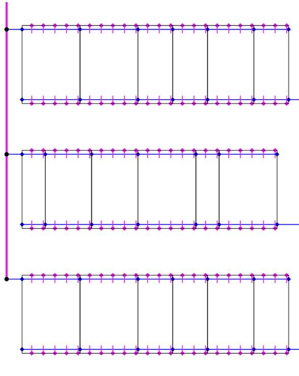
In the routing channels between the cells we route metal1 horizontally and metal2 vertically.
