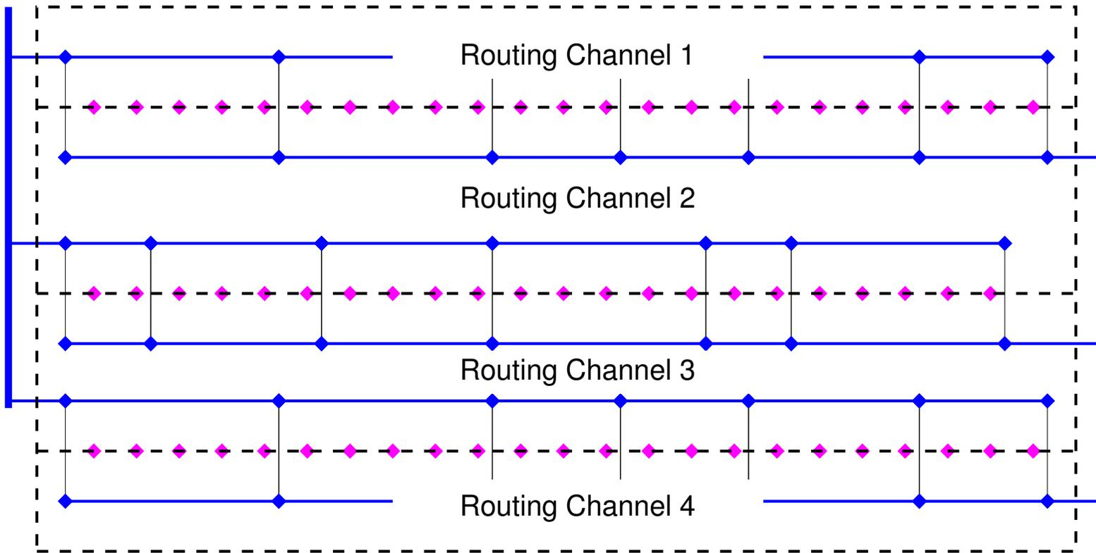
With this approach we can route safely over the cell to the specified pins leading to much smaller gaps between cell rows.
