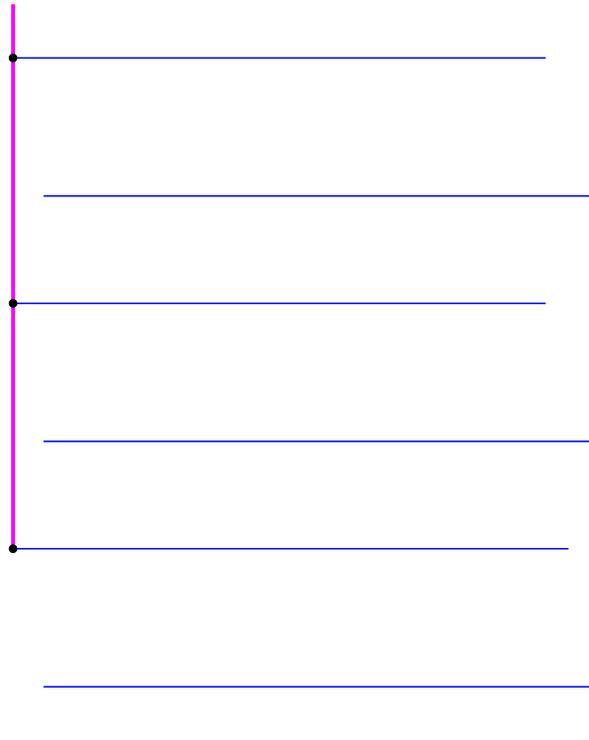
Cells are placed in one or several equal length lines with inter-digitated power and ground rails.
