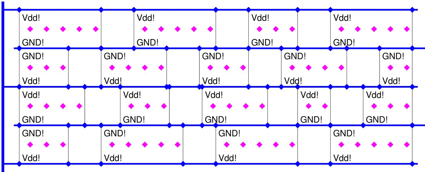
By flipping every second row it may be possible to eliminate gaps between rows. N-wells are merged and power or ground rails are shared. This approach is normally associated with sparse rows and non channel based routing algorithms.
