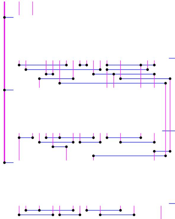
In the routing channels between the cells we route metal1 horizontally and metal2 vertically.
