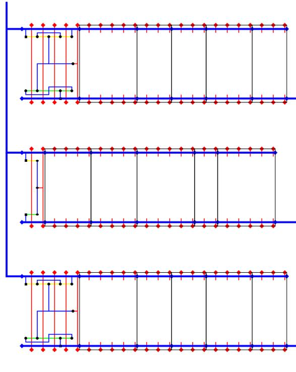
Inter-digitated power and ground rails can be routed using only one metal layer.<sup>1</sup>
