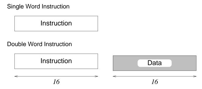
The data word contains either the operand itself (immediate addressing mode) or a value which will be used to calculate the operand address in memory.
