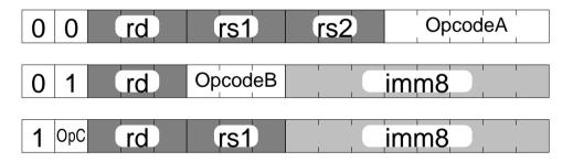
**OpcodeA** allows for up to 32 Register-Register Arithmetic/Logic instructions. **OpcodeB** allows for up to 8 Register-Immediate Arithmetic/Logic instructions.
