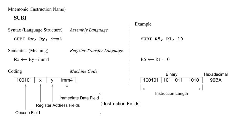
The *instruction set* for a processor is the set of all the instructions supported by that processor.
