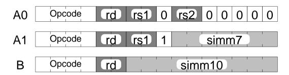
In this case up to 16 instructions are supported, each of which supports either coding A (i.e. A0 and A1) or coding B.
