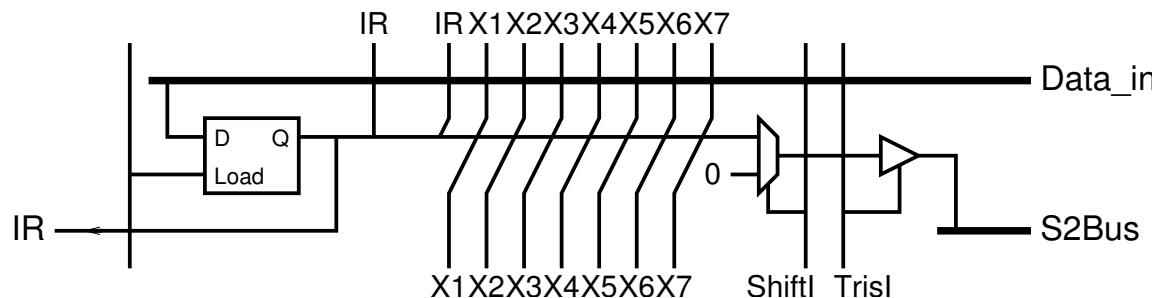
Both bitslices include wiring for 8 bit shift left. **IR\_LO** feeds values into the shifter while **IR\_HI** takes values from the shifter.
