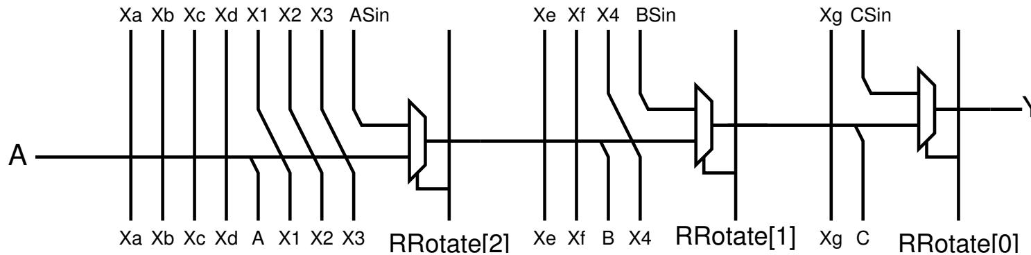
N.B. Most single bit rotate functions will *rotate through the carry*. This barrel rotation, based on the SPARC implementation, does not make use of the carry for input or output.
