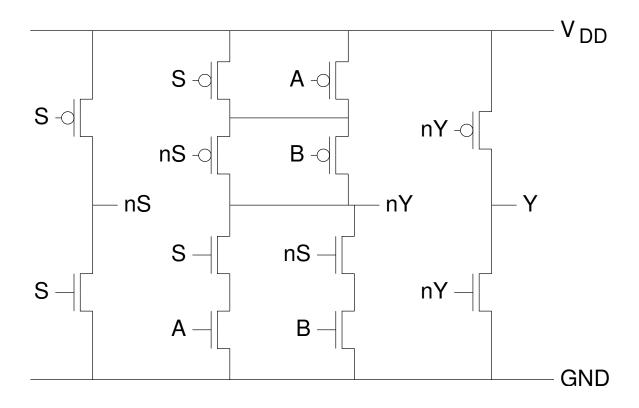
a circuit diagram where all the elements are transistors
