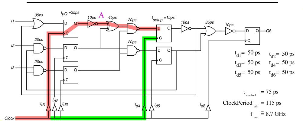
$$ClockPeriod > t_{pQ} + t_{comb-A} + t_{setup} + (t_{d1} - t_{d4})$$
