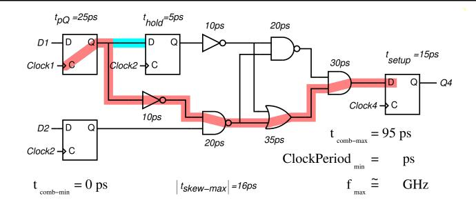
• What is the maximum operating frequency of the circuit if the clock skew is no more than 16ps?
