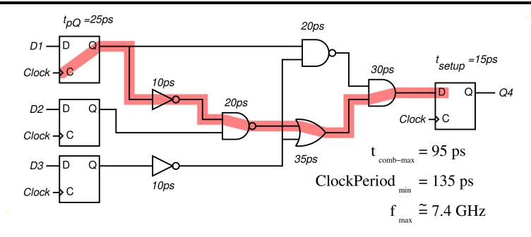
• Critcal path analysis allows us to determine the maximum feasible clock frequency:
