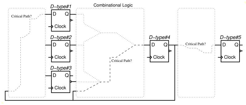
$$ClockPeriod > t_{pQ} + t_{comb-crit} + t_{setup} + (t_{d_{launch}} - t_{d_{capture}})$$
