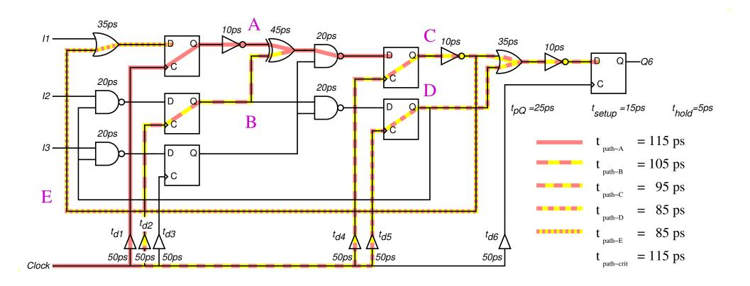
$\Rightarrow$  Initially try increasing  $t_{d4}$  by 20ps
