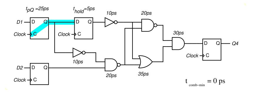
$$t_{pQ} + t_{comb-min} > t_{hold}$$
