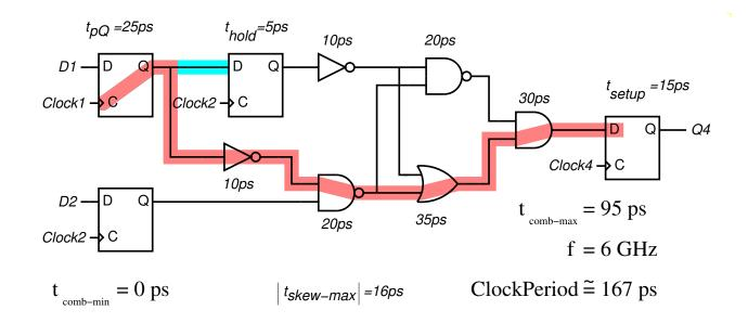
• What is the maximum jitter that can be tolerated given an operating frequency of 6GHz and clock skew of no more than 16ps?<sup>6</sup>
