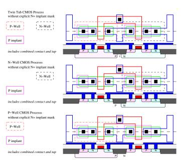
Twin Tub CMOS Process without explicit N+ implant mask N-Well P-Well P implant includes separate contact and tap N-Well CMOS Processs without explicit N+ implant mask N-Well P implant includes separate contact and tap P-Well CMOS Processs without explicit N+ implant mask P-Well ---┝╟═╌ P implant includes separate contact and tap 4103
