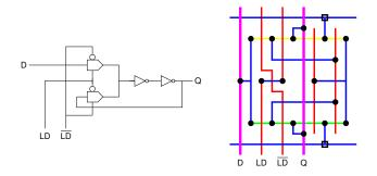
– a compact layout is possible using 2 layer metal
