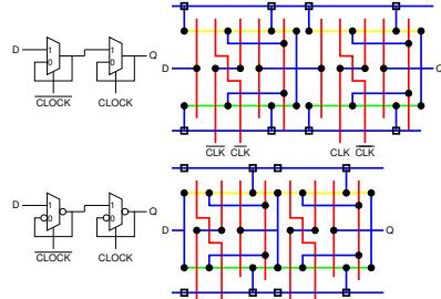
\*multiplexor based latches and flip-flops include distinctive polysilicon crossover
