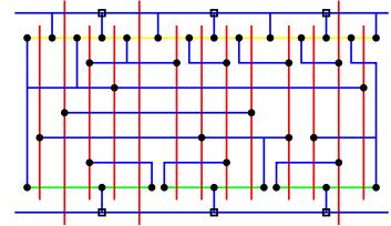
Euler path analysis is applied creatively to these multi-gate cells – gates are often linked via the common gnd/pwr node
