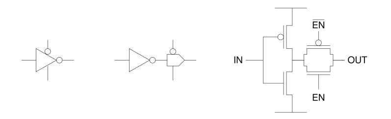
Any gate may have a tri-state output by combining it with a transmission gate.
