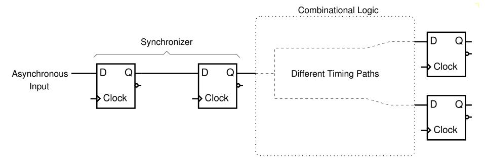
A second flip-flop in the synchronizer gives a predictable  $t_{pQ}$  for our equation:
