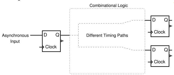
Retiming the asynchronous input before the combinational logic block should give more predictable results.
