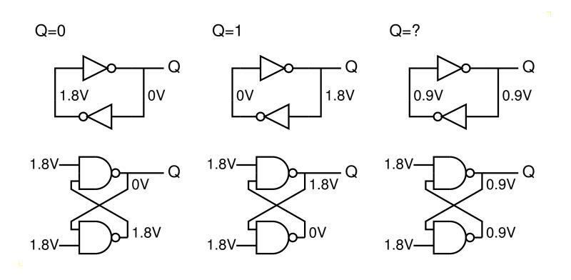
The third state is described as *metastable* since a slight perturbation in one of the 50%-of- $V_{DD}$  voltages will result in a move to one of the other states.
