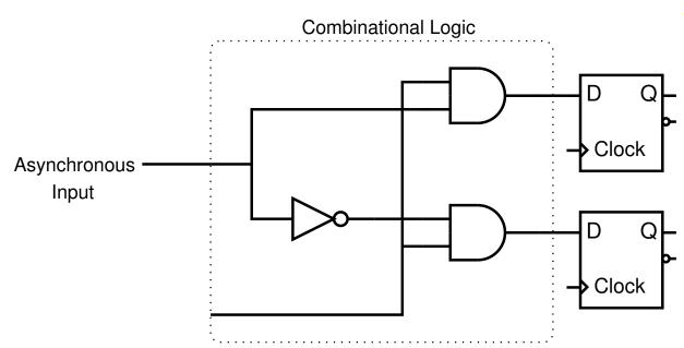
With different timing paths through combinational logic, we can get unexpected results.
