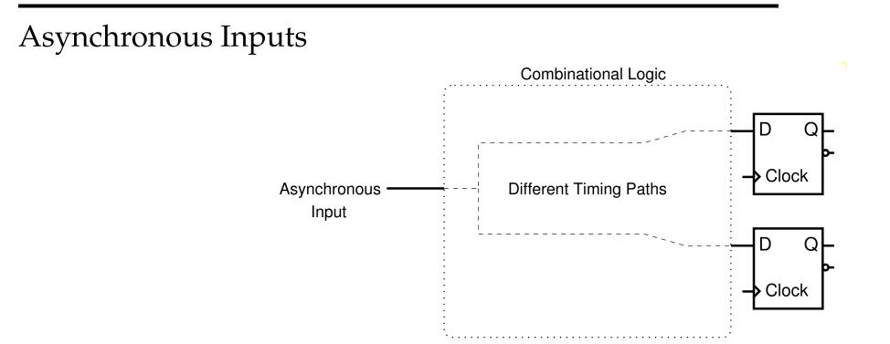
With different timing paths through combinational logic, we can get unexpected results.
