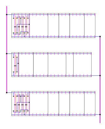
Cells are placed in one or several equal length lines with inter-digitated power and ground rails.
