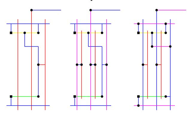
Most modern VLSI processes support two or more metal layers. The norm is to use only metal for inter-cell routing. Either Metal1 horizontally (and for power rails) and Metal2 vertically (and for cell inputs and outputs) or vice versa.
