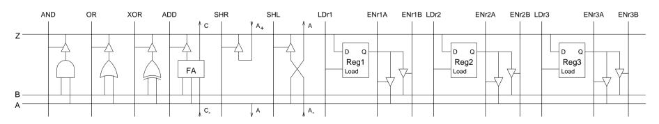
• Bit Sliced Datapath Right Shift Left Shift Out Carry Out AND XOR ADD SHR SHL LDr1 ENr1A ENr1B LDr2 ENr2A ENr2B LDr3 ENr3A ENr3B Z[3] Reg2 Reg1 Reg3 FΑ B[3] -A[3] C<sub>-</sub> Z[2] Reg1 Reg2 Reg3 FΑ Load Load Load B[2] A[2] Z[1] Reg1 Reg2 Reg3 Load Load Load B[1] -A[1] C<sub>-</sub> Z[0] Reg1 Reg2 Reg3 Load B[0] A[0] C\_ Carry In Right Shift Out Left Shift In
