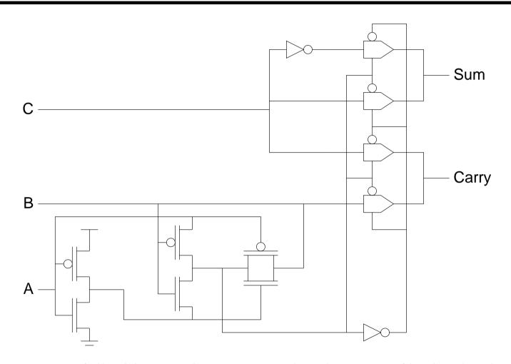
An 18 transistor full adder may be constructed making use of both XOR designs.
