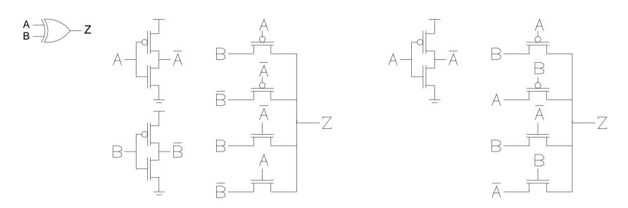
The first design employs a transmission gate multiplexor while the second is the standard 6 transistor XOR:
