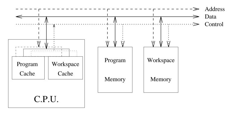
• The separate caches appear to allow access to workspace and program memory in the same cycle.
