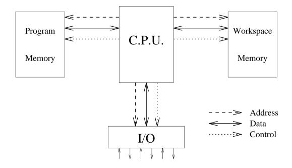
• The Harvard Architecture uses different sets of buses for different components.<sup>1</sup>
