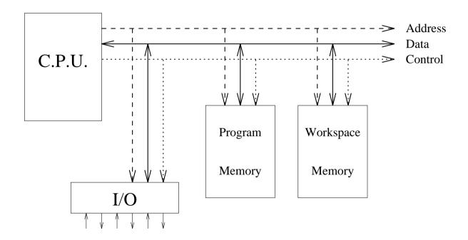
• The Princeton Architecture uses a common set of buses for all components.
