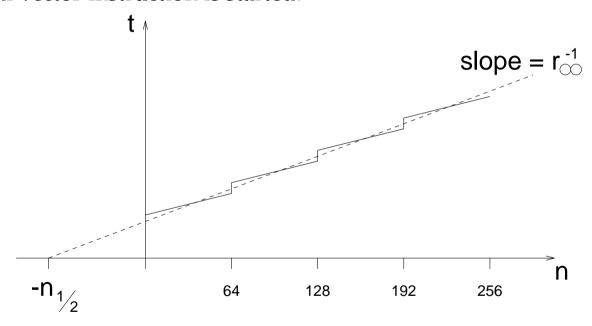
The solid line indicates the actual performance while the dashed line indicates the equivalent generic performance, a best fit line giving values for  $r_{\infty}$  and  $n_{1/2}$ .
