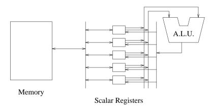
The memory may typically take three processor cycles for a single transfer while the A.L.U. may consume two values and produce one for every arithmetic operation.
