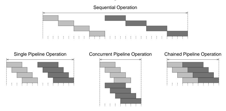
• Sequential Operation. *no pipeline*No operation is started until the previous result has been obtained.
