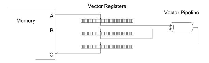
Where more than one pipeline is concurrently active, the architecture relies on the use of local register values to maintain the power bandwidth balance.
