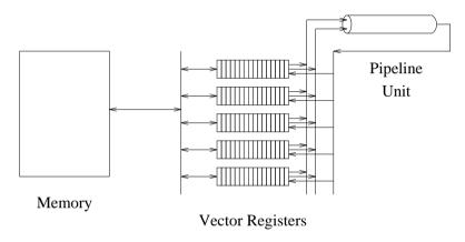
In the case of the pipeline processor we are aiming to calculate a new result every clock cycle.
