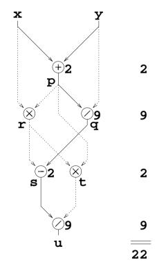
Our simple control flow description does not exploit the early availability of  ${\bf r}$  in order to take  ${\bf t}$  out of the critical path. If we produce a dataflow machine based on execution of the dataflow graph we can exploit the full parallelism with ease.
