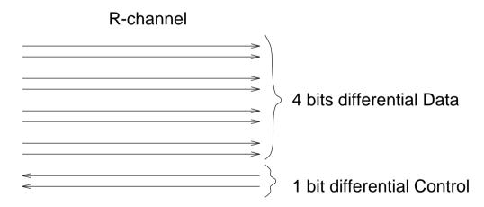
• Communication is synchronous - all PEs and routing nodes share the same clock!
