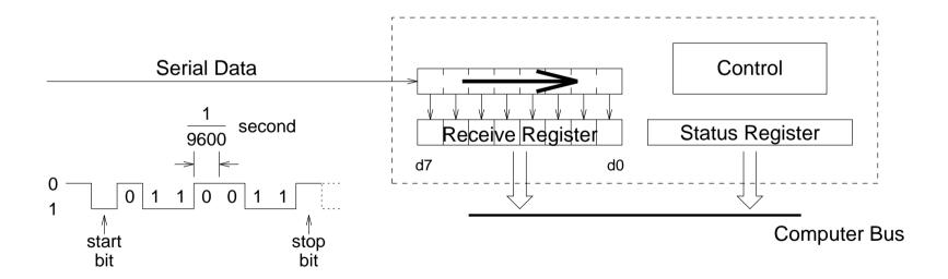
Data must be extracted from the receive register before the next byte is received.
