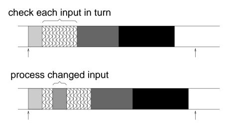
Before recalculating the flight parameters, we poll each input in turn to check if it has changed. Changed inputs require input processing.
