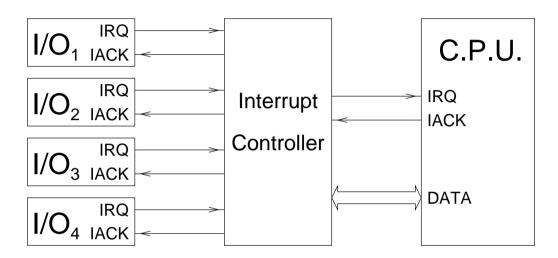
External interrupt controllers are used where we wish to deal efficiently with large numbers of I/O devices.
