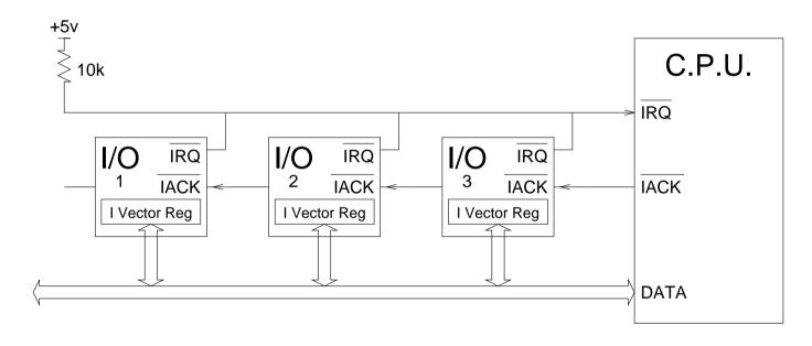
• An alternative strategy allows the I/O device to identify itself during the IACK cycle.
