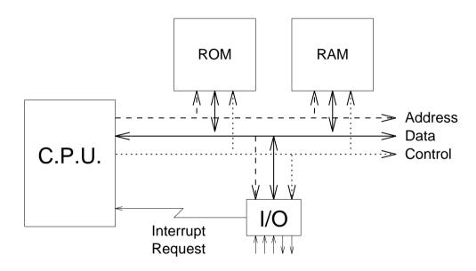
The assertion of the interrupt request line by an I/O device should initiate an interrupt cycle.
