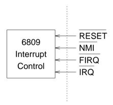
The simplest is the Fast Interrupt Request line,  $\overline{FIRQ}$ . We shall consider the interrupt cycle initiated by asserting  $\overline{FIRQ}$ .
