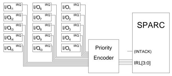
• A more advanced system might use a custom interrupt controller combined with the INTACK signal from the SPARC<sup>2</sup>.
