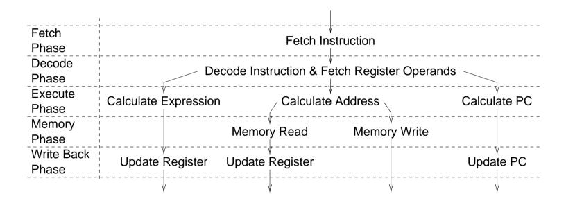
No unit is used more than once for each instruction<sup>1</sup>, the whole instruction may be completed in a *single clock cycle*.
