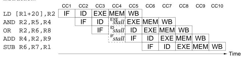
In the  $4^{th}$  cycle the EXE stage is *stalled* in order to avoid a *load-use* hazard. In turn this stalls IF & ID while MEM (& WB) are allowed to continue. The result is a *bubble* in the pipe which appears in the MEM stage in the  $5^{th}$  cycle. It is not possible to show this *bubble* on an instruction oriented pipeline diagram.<sup>8</sup>
