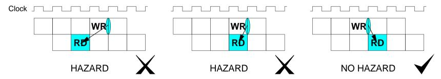
A *Read after Write* hazard is caused by a *True Dependency* since the second instruction *depends* on the result of the first.
