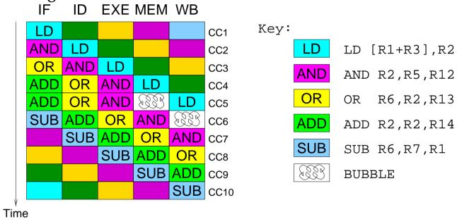
Here it can be seen that the *bubble* is simply an empty pipeline stage which arises when the AND instruction is stalled while the LD instruction continues. Once created a *bubble* will usually advance through the pipe until it reaches the last stage as if it was a normal instruction. In the  $6^{th}$  cycle we see the *bubble* in the WB stage.
