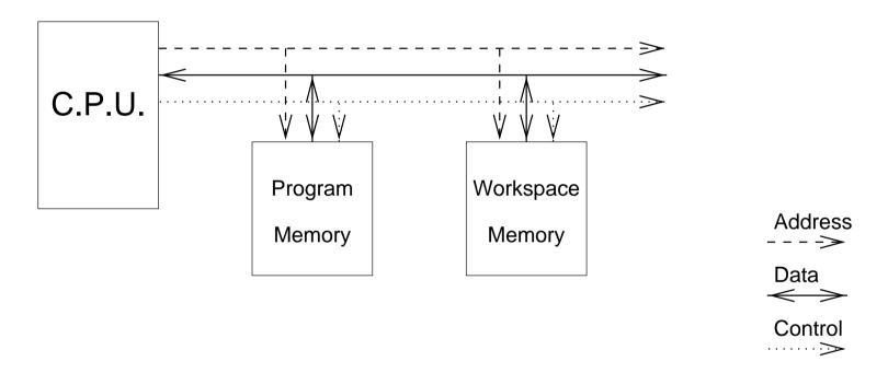
• The Princeton Architecture uses a common set of buses for all components.
