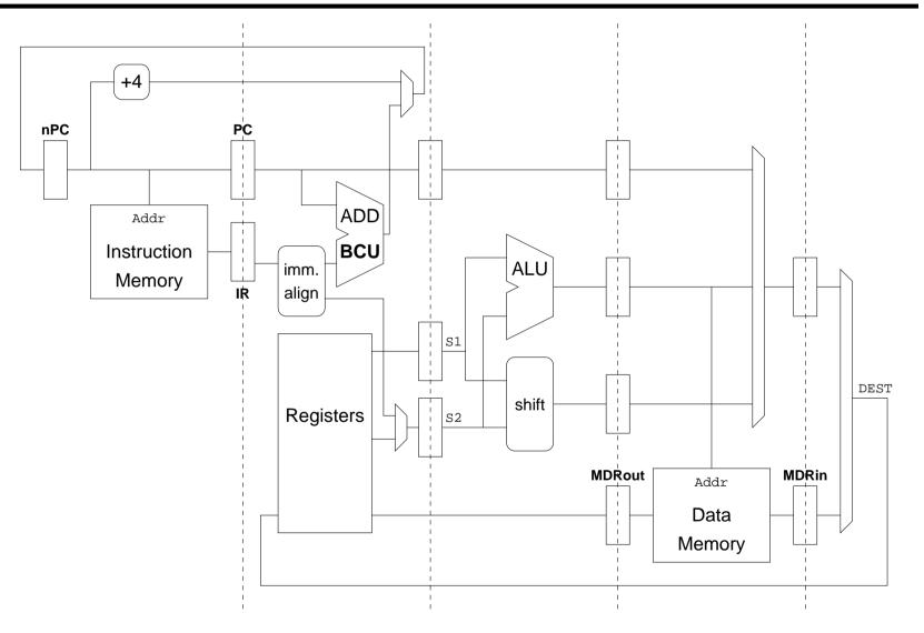
This technique of flushing instructions when a branch is taken is actually a simple form of branch prediction:
