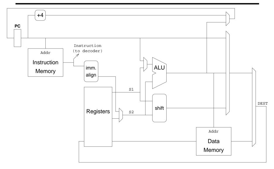
To support a throughput of 1 instruction every cycle we must ensure that no bus or functional unit is used more than once in the instruction cycle.
