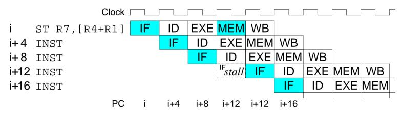
• The data access is given priority and the instruction fetch must be stalled.
