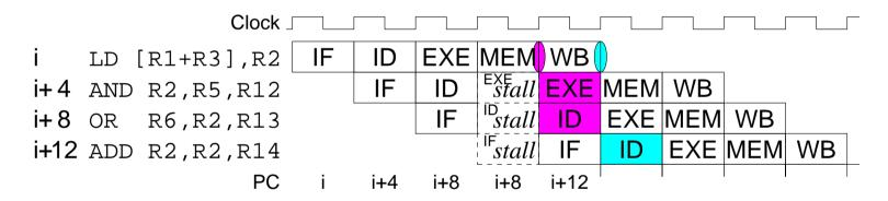
Although some machines support a *delayed load*, where the new value is unavailable for the next instruction, the SPARC requires a single cycle stall in order to maintain assembly language semantics<sup>7</sup>.
