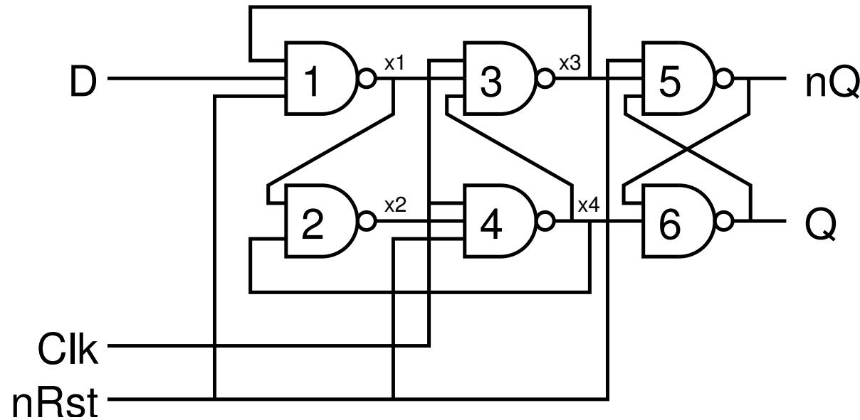
Here each NAND gate is allocated a different pair of rows in the layout (further optimization of this circuit is possible).
