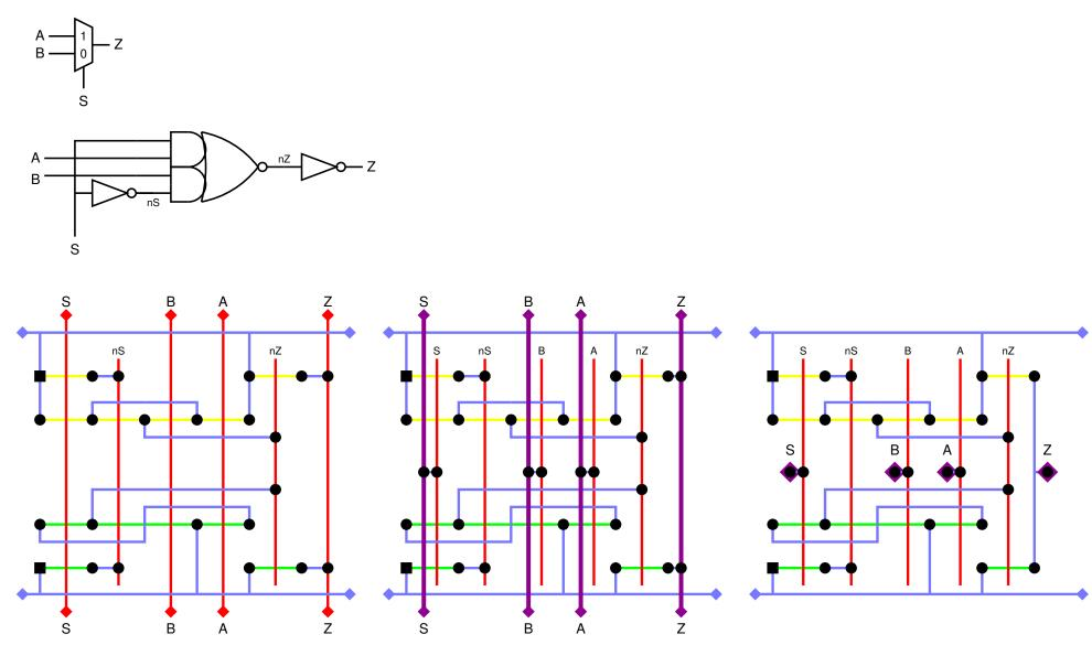
Gate Matrix Style Mux – (for processes with one, two or three metal layers)
