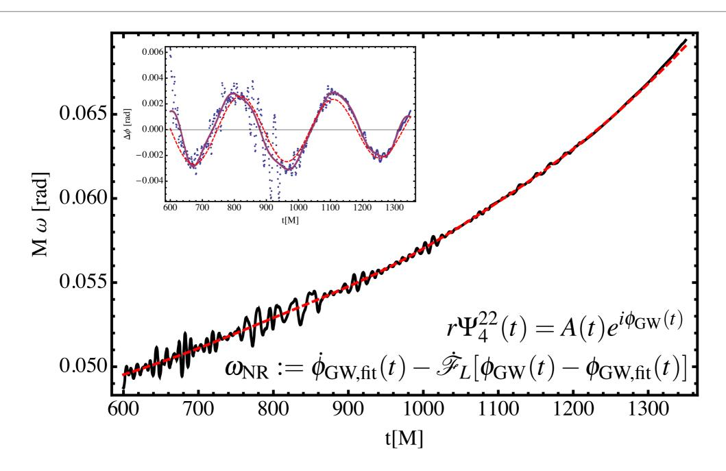
A combination of fitting and filtering methods is used to produce a cleaned GW frequency while preserving the delicate eccentricity oscillations.
