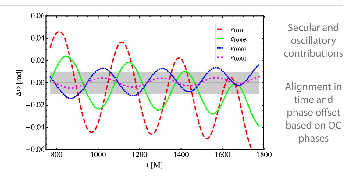
Phase differences from  $\Psi_4$  with respect to the  $e_{\phi, \rm GW} = 0.0003$  simulation. A stringent NR phase error requirement of ±0.01 rad is indicated by the shaded region.
