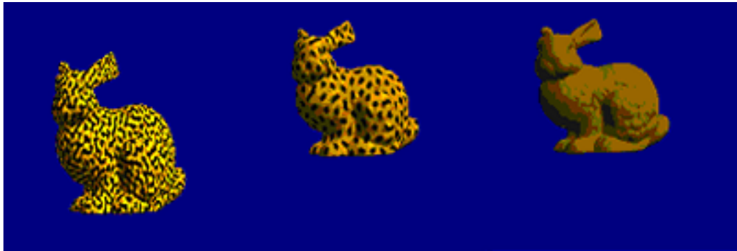
FIGURE 6.3: (a) reduced the activator's diffusion rate ( DA ), (b) reduced the inhibitor's diffusion rate ( DI = 0.2 ), (c) further reduced the inhibitor's diffusion rate ( DI = 0.15 ), R-D cannot continue.
