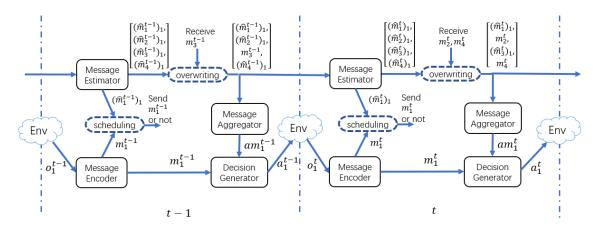
Figure 1: The demonstration of the proposed MBC framework, including the decision making process of one agent at time step t-1 and t in a four-agent MARL system. In addition to the notations mentioned in Section 3,  $(\hat{m}_j^t)_i$  represents agent j's message at t estimated by agent i.
