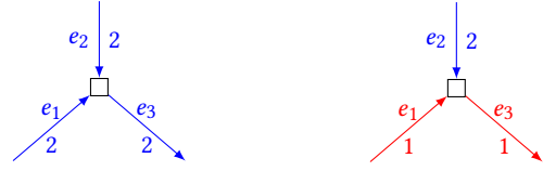
Figure 4: The two types of nodes in an AND/OR graph: OR node (left) and AND node (right). An OR node has three incident edges of weight 2 (blue), while an AND has two incident edges of weight 1 (red) and one of weight 2.
