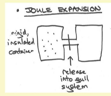
No work is done on surroundings W=0 Adiabatic so Q=0 => the internal energy U is unchanged
