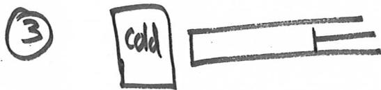
$C \rightarrow D$ : in contact with cold reservoir isothermally compress.
