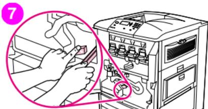
7 Hold the tab down and use the tongs (found in the inside pocket of the right front door) to reach into the printer and remove jammed media. Make sure to remove any pieces of torn media.
