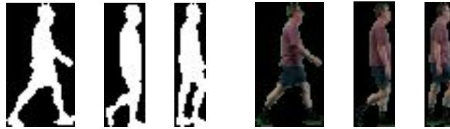
(c) The connected region is isolated and a mask created. This is used directly for the greyscale signature (d) The connected region is isolated and a mask created. This is used to extract the individual for the colour signature
