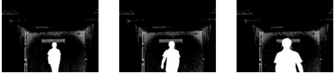
(b) Each frame of the walk has the background subtracted. The largest connected region is taken as being the subject
