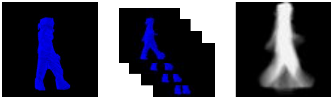
(c) Using each silhouette, volumetric carving is used to construct a model (d) The model of each frame is used to capture a silhouette from a novel perspective (e) These silhouettes are combined to produce a single signature
