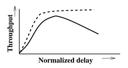
Better performance can be achieved if user continues to listen to medium while transmitting and stops transmission immediately if collision is detected  $\Rightarrow$  CSMA with collision detection
