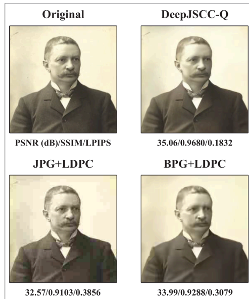
FIGURE 4. Rydberg wireless communication experimental results of the image transmission performance using PSNR, SSIM, and LPIPS for evaluation.
