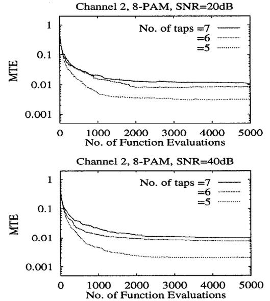
Figure 4. Mean tap error versus number of function evaluations for channel 2.
