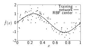
5-term model mapping (curve) produced by the combined LROLS and Doptimality algorithm with  $\beta=10^{-5}$  for simple scalar function modelling problem. Dots indicate noisy training data y and circles the RBF centers.
