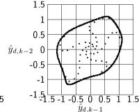
Comparison of underlying noise-free system  $y_{d,k}$  and iterative RBF model output
