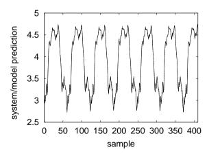
Comparison of system output  $y_k$  and model one-step prediction  $\hat{y}_k$ . 22-term model produced by combined LROLS and D-optimality algorithm with  $\beta=10^{-5}$
