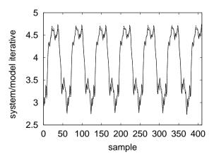
Comparison of system output  $y_k$  and model iterative output  $\hat{y}_{d,k}$ . 22-term model produced by combined LROLS and D-optimality algorithm with  $\beta=10^{-5}$
