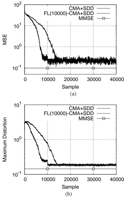
Fig. 9. Convergence performance comparison of the CMA+SDD and FL(10000)-CMA+SDD, in terms of: (a) the MSE and (b) MD measure, averaged over 10 runs and given SNR= 38 dB. The FL(10000)-CMA uses the fuzzy step size for the first 10000 samples and then switches to a constant step size.
