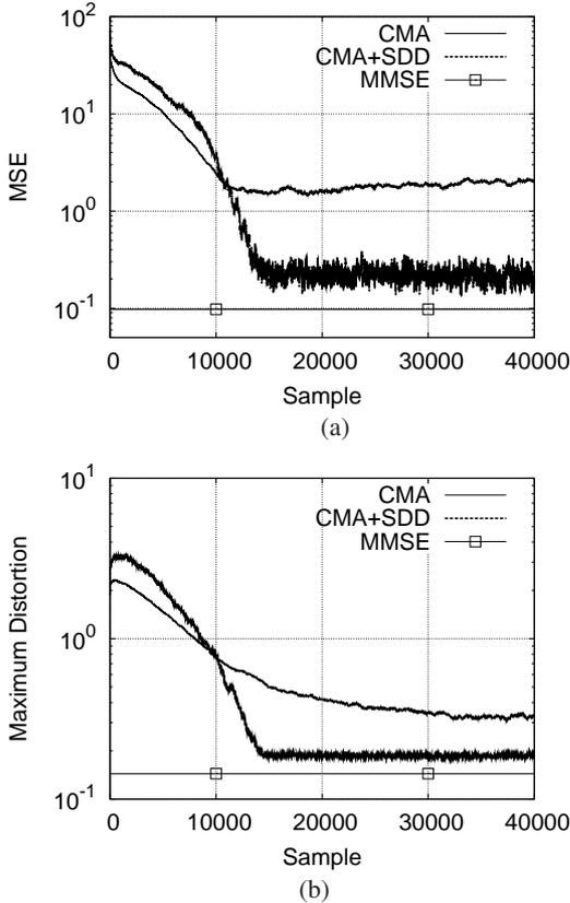
Fig. 5. Convergence performance comparison of the CMA and CMA+SDD, in terms of: (a) the MSE and (b) MD measure, averaged over 10 runs and given SNR = 38 dB.
