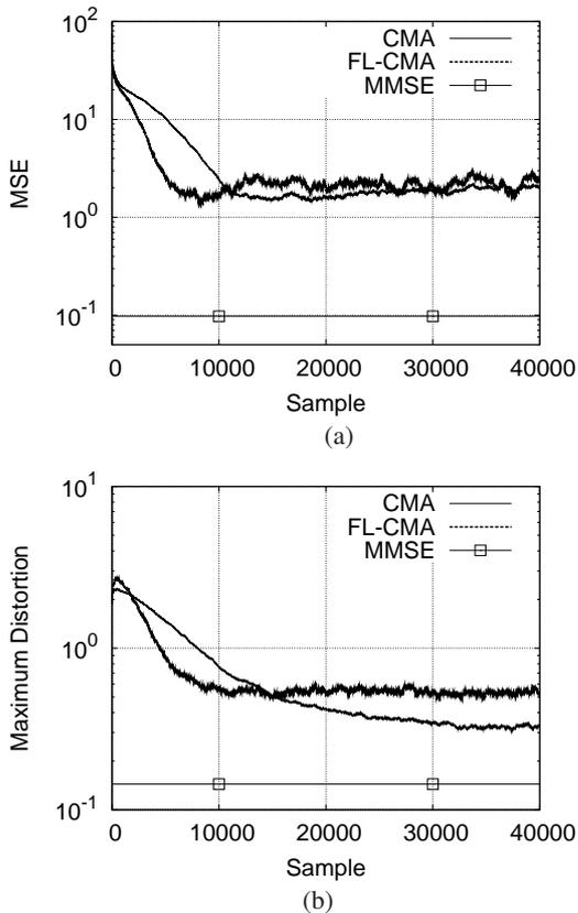
Fig. 7. Convergence performance comparison of the CMA and FL-CMA, in terms of: (a) the MSE and (b) MD measure, averaged over 10 runs and given SNR= 38 dB.
