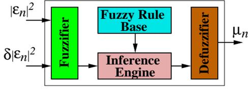
Fig. 1. Schematic of the fuzzy inference system for tuning the step size of the CMA. The operational rate  $n$  of the FIS is  $N_{sm}$  times slower than the symbol rate  $k$ .
