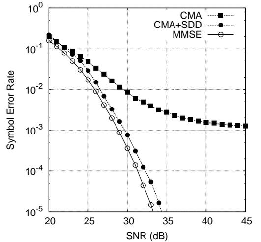
Fig. 6. Symbol error rate comparison of the three equalisers.
