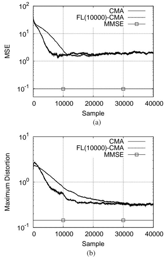
Fig. 8. Convergence performance comparison of the CMA and FL(10000)-CMA, in terms of: (a) the MSE and (b) MD measure, averaged over 10 runs and given SNR= 38 dB. The FL(10000)-CMA uses the fuzzy step size for the first 10000 samples and then switches to a constant step size.
