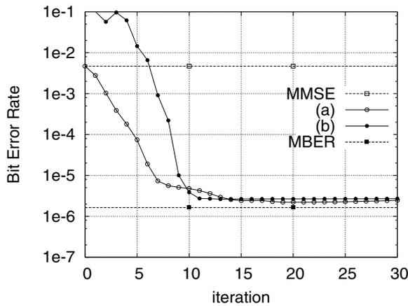
Fig. 3. Convergence rate of the block-data gradient adaptive MBER algorithm with  $K = 400$ , SNR= 17 dB,  $SIR_2 = SIR_3 = 0$  dB and  $SIR_4 = -6$  dB, and given (a): initial  $\mathbf{w} = \mathbf{w}_{MMSE}$ ,  $\mu = 0.3$  and  $\rho_n^2 = 0.06$ ; and (b): initial  $\mathbf{w} = [0.0 + j0.1 \ 0.1 + j0.0 \ 0.1 + j0.0]^T$ ,  $\mu = 0.7$  and  $\rho_n^2 = 0.06$ .
