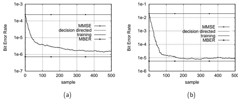
(a):  $SNR = 10$  dB,  $SIR_i = 0$  dB for  $i = 2, 3, 4, 5$ ,  $\mu = 0.03$  and  $\rho_n^2 = 8\sigma_n^2 = 0.4$ .
